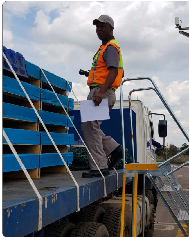
Stepping off the ladder onto the truck is a much safer way than climbing off the ladder on to the truck
