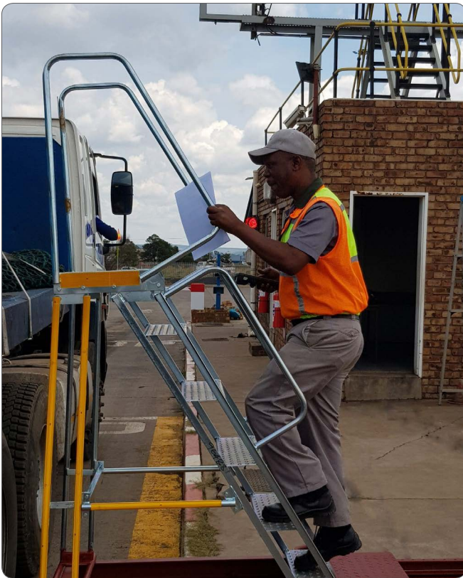
Guard climbing onto modified ladder, to climb onto truck/trailer, free movement of hands
